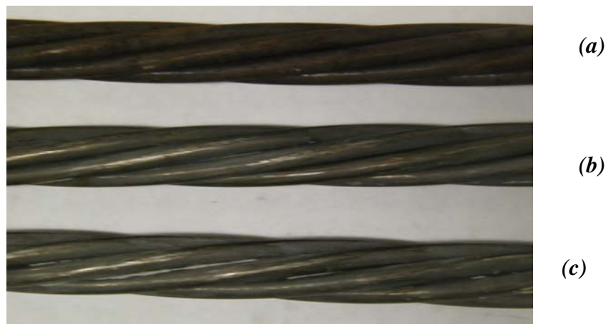
Figure 2-10 Photograph of surface of strands: (a) Strand A, (b) Strand B, (c) Recovered from bending fatigue specimen
