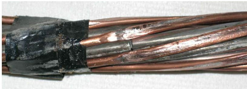
Figure 2-1 Wire break within grip
