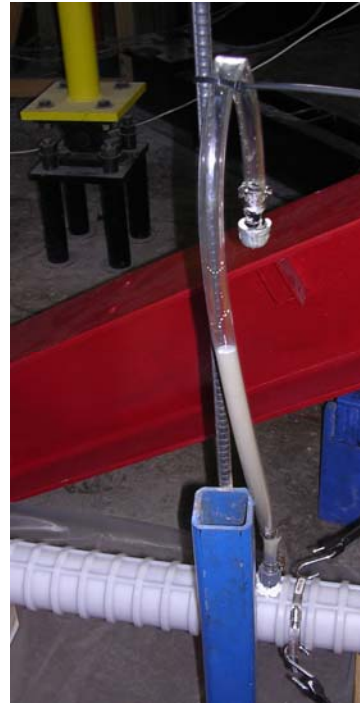
(b) Vent hose after grouting
