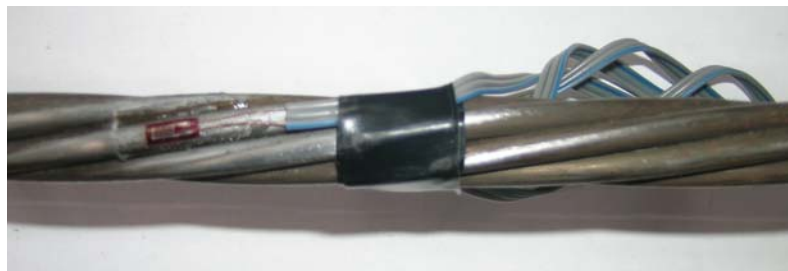
Figure 3-11 Strain gage on strand
