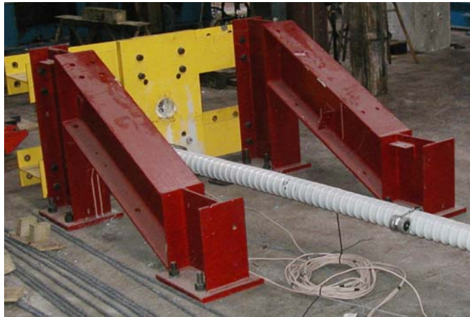
Figure 6-3 North end of Specimen 1 at end of fatigue test
