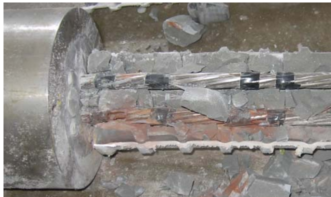
Figure 6-12 Autopsy of specimen 2
