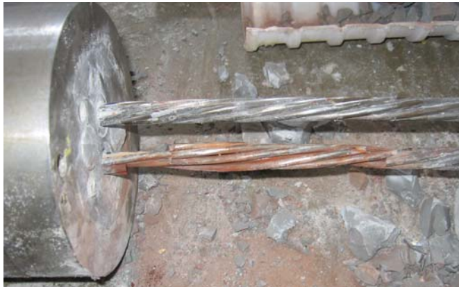
Figure 6-13 Specimen 2 after grout has been removed
