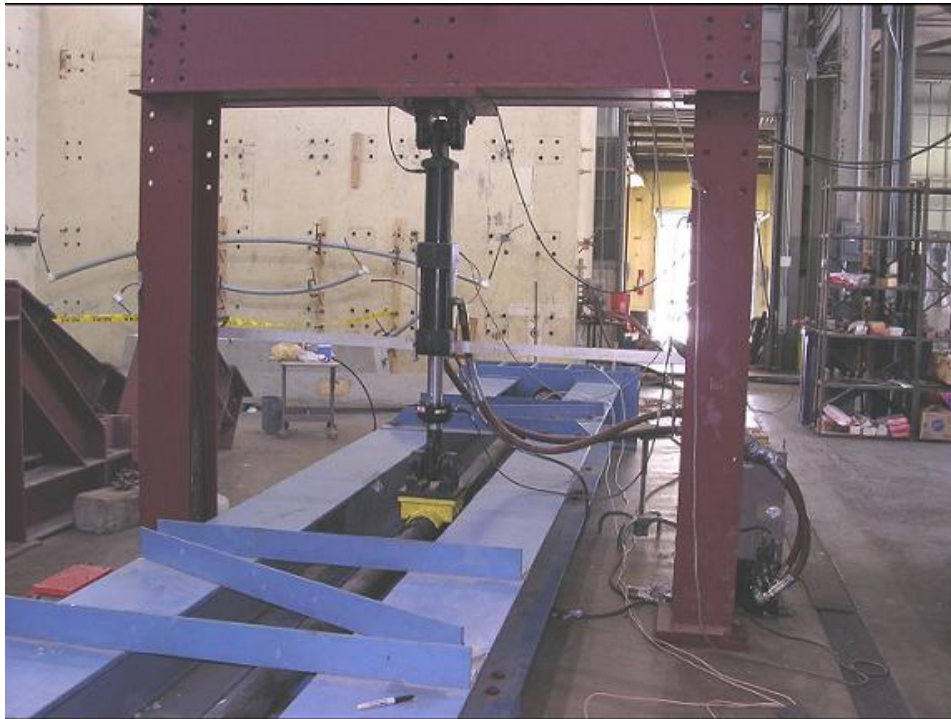
Figure 1-10 Large-scale bending fatigue tests (Ridd, 2004)
