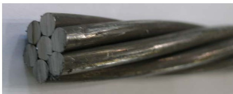
Figure 3-6 0.6-in. diameter prestressing strand
