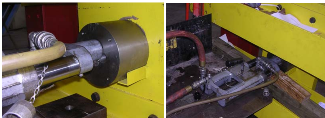
Figure 3-9 Stressing of strands individually with hydraulic ram
