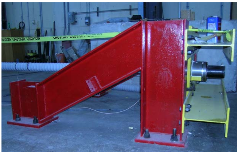
Figure 3-2 Reaction frame and anchor support
