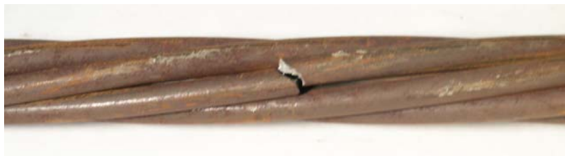
Figure 2-2 Acceptable wire break along free length
