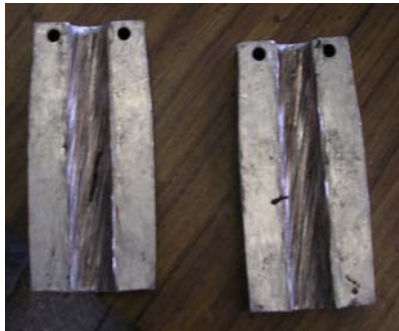
Figure 2-5 Aluminum grips after excessive use
