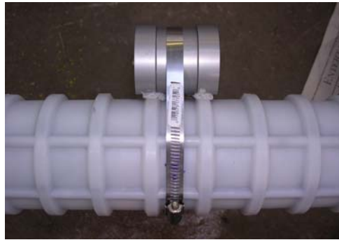
(a) Sensor attached to anchor head (b) Sensor attached along stay length
